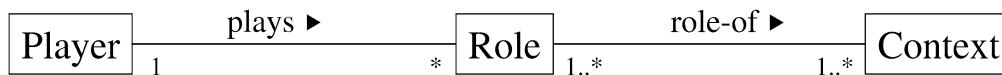
Fig. 1. Basic role model. It relates roles with two recurrent notions from the literature: player and context.
